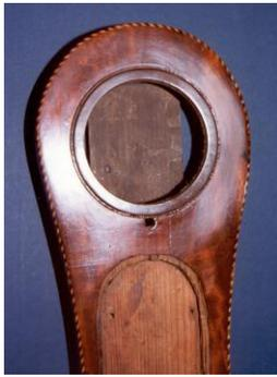
The hygrometer housing at the top was very badly damaged and the bezel and glass missing. I purchased a nice quality ready-made bezel from Barometer World but it was too small in diameter to fill the hole. Therefore I decided to use imagination and after patching in the hygrometer keyhole I made a ring housing as shown on the left. The bezel fits into the hygrometer with a tight push fit. On the back it looks like this -
